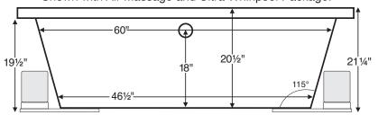
IMPORTANT: Air baths and tubs with a pre-leveled foam base add 2-3" to overall tub height.
