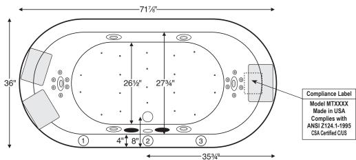
Numbered areas on tub deck represent possible locations to install cleaning systems, faucets and other fixtures. When Fill-Flush is ordered and location 2 is chosen, the detergent feeder will need to be offset to the left or the right.
